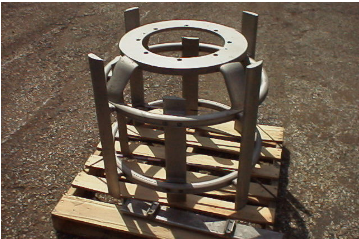
Model 14/40 B Rotating assembly for Bird ( Voith) Centriscreen
